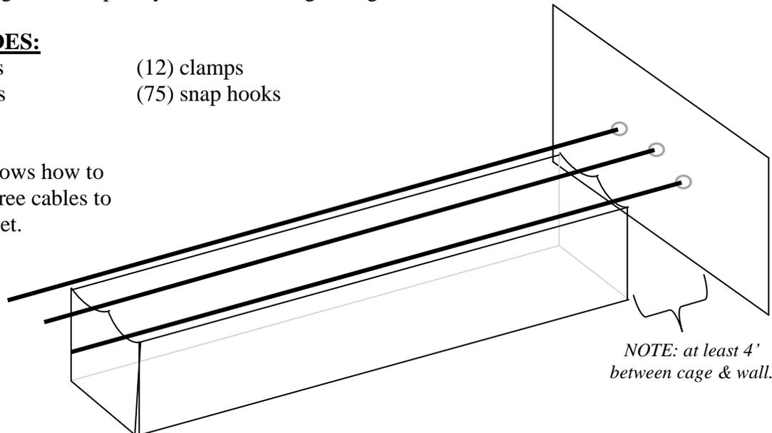
Wall hooks are often installed at the time many gymnasiums are built so they are not included with this kit. A total of six wall hooks or eyebolts are needed for three suspension cables. It is suggested that the center cable be positioned about one foot higher than the outside two cables. This will help keep the ceiling part of your net higher in the center.
